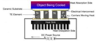
Fig. 1. Schematic Diagram of a Typical Thermoelectric Cooler. Image. March 30 2011. <http://thermal.ferrotec.com/technology/ thermoelectric/thermalRef02/>. Pros: High cooling capacity
