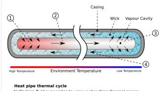
Working fluid evaporates to vapour absorbing thermal energy.
