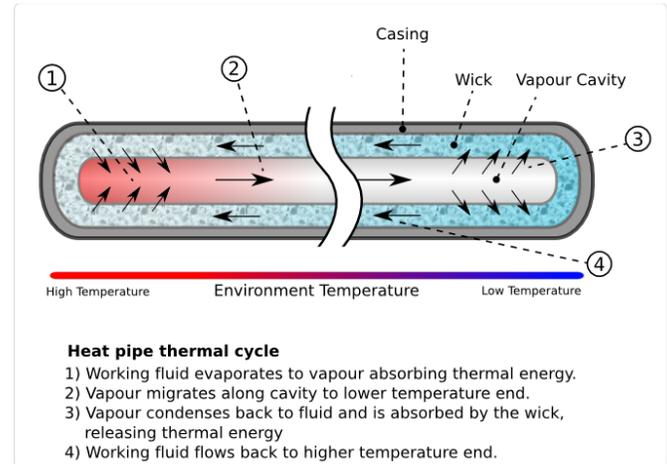
Fig 4. Heat Pipe Mechanism. Image. March 30 2011. < [http://www.techreaction.net/wp-content/uploads/2010/05/Heat\\_Pipe\\_Mechanism.png](http://www.techreaction.net/wp-content/uploads/2010/05/Heat_Pipe_Mechanism.png)>.
